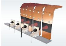
Installation example for IR temperature sensors for contact-free detection of the temperature development at the busbars
